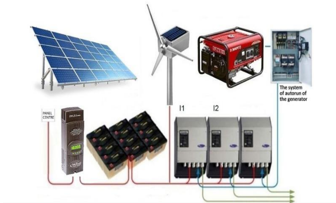
Figure 1. Typical block diagram of off-grid hybrid power plants
